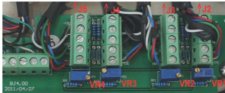
Adjustment of weighing cell J2 takes place at the potentiometer VR1.
